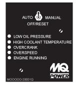
During *cranking cycle*, The MPEC will attempt to crank the engine for 10 seconds before disengaging. If the engine does not engage (start) by the third attempt, the engine will be shutdown by the engine controller's "Over Crank Protection" mode. If the engine engages at a speed (RPM's) that is not safe, the controller will shutdown the engine by initializing the "*Over Speed Protection*" mode.
